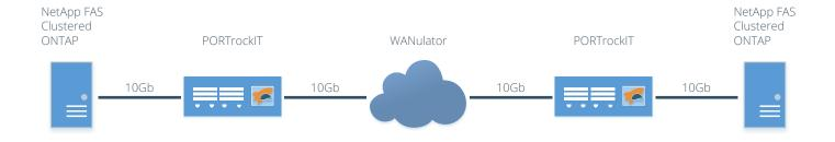
Figure 2: Accelerated architecture with PORTrockIT
